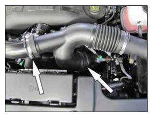
3. Loosen the three hose clamps that secure the factory intake tube and then remove the factory intake tube from the vehicle.
