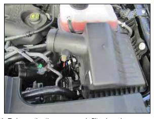
4. Release the three upper air filter housing retaining clips and then remove the upper air filter housing and factory air filter.
