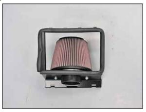
9. Install the  $K\&N^{\otimes}$  air filter onto the filter adapter and secure with the provided hose clamp.
