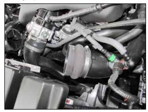
13. Install the provided hump coupler (08418) onto the driver's side turbo inlet tube.
