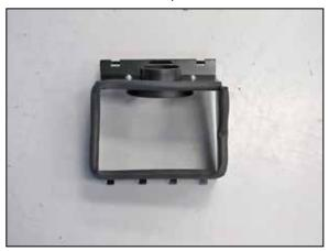
6. Install the "BULB" edge trim onto the top of the  $K\&N^{\scriptsize @}$  heat shield as shown.
