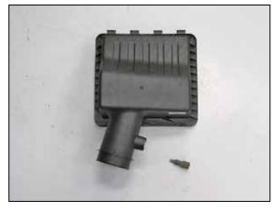
18. Remove the inlet air temperature sensor from the factory air filter housing.
